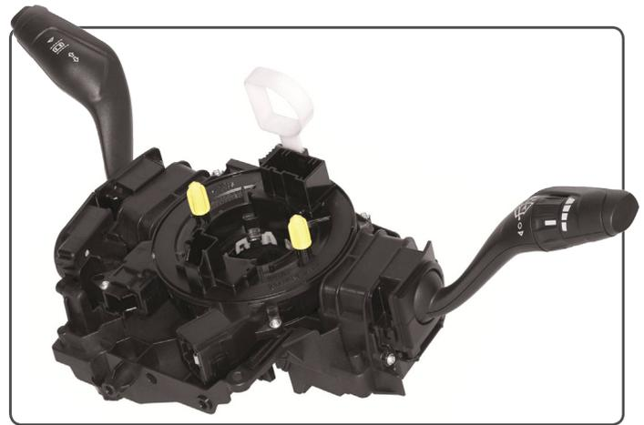
The clock spring is positioned in the center of a typical steering column control module.
